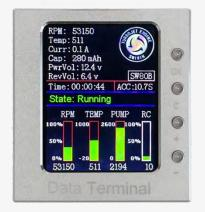
③ after entering the startup mode, the throttle progress bar flashes continuously.
