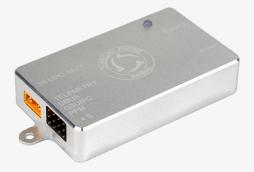
ecu (v3) completes control of engine starting, acceleration and deceleration, steady state, and parking based on input control commands. under actual flight altitude, flight speed, and climate conditions, the ecu (v3) adjusts the fuel supply of the oil pump to maintain stable engine operation at a certain speed.
